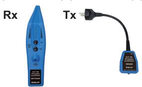
The Transmitter (Tx) draws a current from the mains supply circuit to which it is connected to. The Signal Current from the Tx is at about 10kHz. The Transmitter is powered by the mains and requires no batteries.
